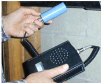
Hand probe detects ultrasonic leaks.
