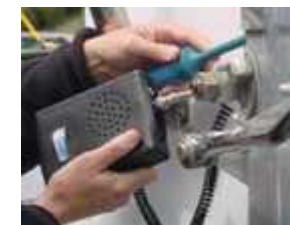
Rubber sound concentrator slips over end of hand probe to pinpoint leak location.
