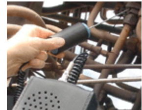
Contact probe locates mechanical malfunctions.
