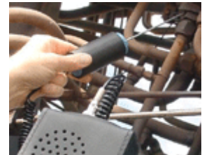
Contact probe locates mechanical malfunctions.
